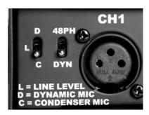
Select "48PH" microphone power or "DYN" by selecting the switch located next to each input XLR connector. Only select "48PH" when using microphones designed to operate from 48PH or 9-52PH or 9-52 simplex power. For all other uses, select "DYN".
