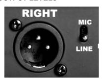
The output XLR's can be set to either microphone level "MIC" or to line level "LINE". This level must match the input level of your camera. See your camera's owner's manual for proper level selection. When in doubt, set the DV Promix 3's outputs to "MIC" and try it. If you find the audio level to be very low or non-existent, then set the switches to "LINE".
