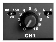
For use indoors, or outdoors with no wind present, select "20". For outdoors with light wind conditions, select "80". For outdoors with high wind conditions, select "150".
