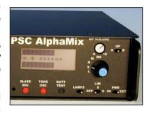
fiber optic light transmission panel with a high performance "green" LED as a light source rather than an electro-luminescent system. The combined approaches yield quality backlighting without introducing noise. To activate the lamps there is a toggle switch located below the bottom right corner of the meter.
