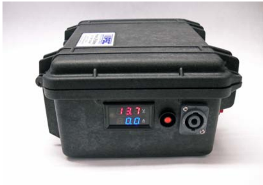
Side View Showing Volt and Current Meters
